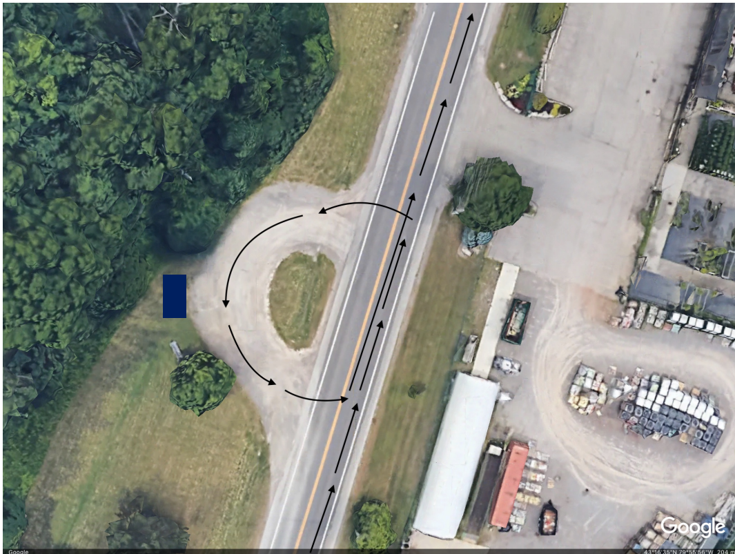
Figure 3: Depiction of eastbound 15 GO Bus route along Watsons Lane Loop. The blue rectangle represents the passenger platform.
